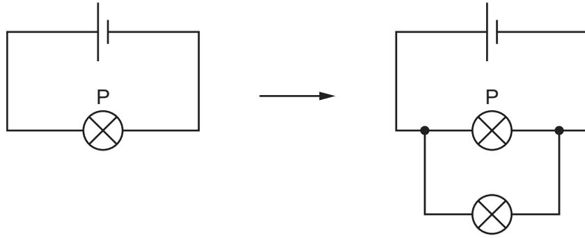
How does this change affect the brightness of lamp P and how does it affect the current in the cell?
